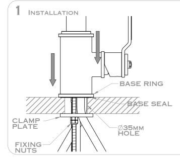
• ENSURE THE BASE SEAL IS IN POSITION BETWEEN BASE RING AND WORKTOP. ENSURE THE TAP IS ORIENTATED TO THE DESIRED POSITION AND THAT
